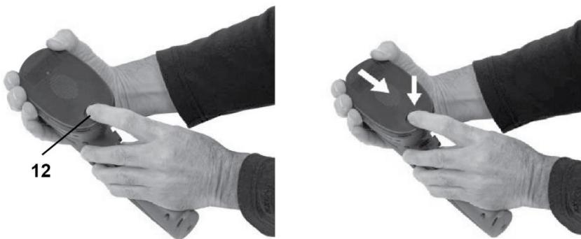
Mount the blade grass (14) trimmer blade (15) so that the two guide pins of the transmission are received in the guide holes of the blade.
